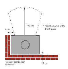
For »elements« with or without lateral extension elements, the above mentioned safety distance to **non combustible elements** and walls (such as concrete, stone, plaster) should be observed.
