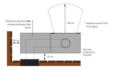
Extension elements, through which smoke discharge tubes are fed can be installed at a distance of at least 30 cm to combustible elements or walls (please observe the DIN of the smoke discharge tubes).
