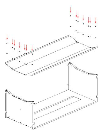
Lastly fasten the top plate to the side plates. Make sure all the plates fit together and that there are no gaps visible between the plates. Fasten all the screws tightly. Your Firebox is now ready to be installed.
