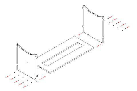
Place the base plate flat and fix the side plates to the base plate with the fasteners and washers provided. Do not tighten the fasteners completely. Hand fasten only as you might need to make a positioning and adjustments when the other plates are attached.
